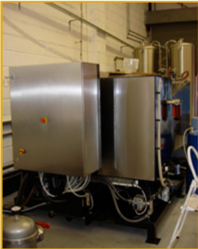
Manufactures 5000 gallons of commercial grade biodiesel per day
